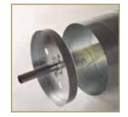
12" diameter drums allow for lower headroom requirements. An enclosed barrel houses the dead axle assembly and protects the factory lubricated springs from direct contact with environmental elements. The inherent strength provided by the spiral barrel minimizes axle deflection providing smoother operation. Because the curtain is attached by screws and not seamed to the barrel, replacement of either independent assembly is cost-effective, quick and easy.
