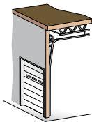
HIGH LIFT break-away is standard, straight incline is available
