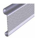
No.  $17 - 2^{"}$  Flat-faced slat up to 22-gauge steel, 22-gauge stainless steel, or 16 B&S gauge aluminum (clear, or bronze anodized). Depth:  $1/2^{"}$ ,  $1-7/8^{"}$  on centers. Secur-Vent<sup>®</sup> – Slat consists of <sup>1</sup>/16"diameter hole offering 20-25% open area over length of each slat. Available in galvanized steel and stainless steel.
